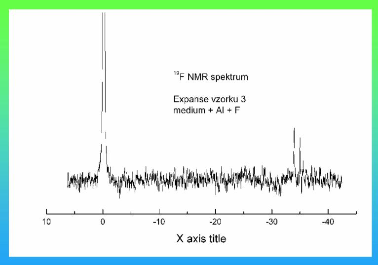
First peak represents free fluoride. Chemical shift of free fluoride was taken as zero and the peaks at - 34 ppm were identified as an alumino-fluoride complexes.
